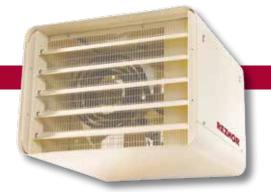
Model EGHB is designed for areas requiring a high level of air flow. This unit heater may be mounted horizontally (wall or ceiling) using supplied brackets or vertically using 4 threaded rods.
